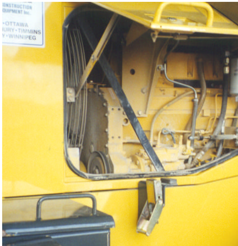
Mount location with auxiliary drive pulley showing.
